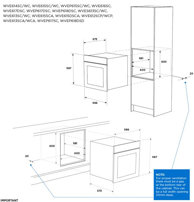
These dimensions are a guide only. All measurements are in millimetres (mm). For complete installation instructions, refer to the manual provided with product.
